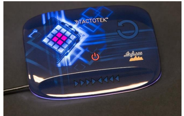
3D in-mold human-machine interface for e.g. automotive applications with printed touch-interface
