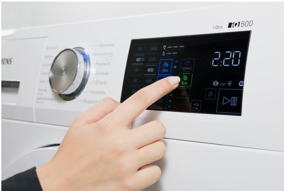
PolyTC sensor film in a series-production white goods touch panel application (Photo: PolyIC)
