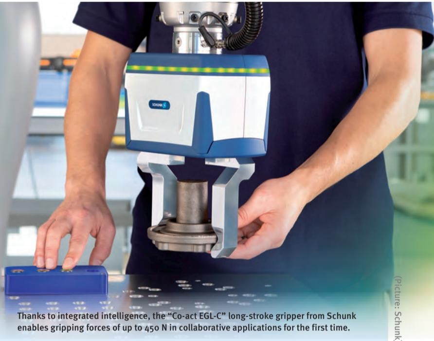
Thanks to integrated intelligence, the “Co-act EGL-C” long-stroke gripper from Schunk enables gripping forces of up to 450 N in collaborative applications for the first time.
