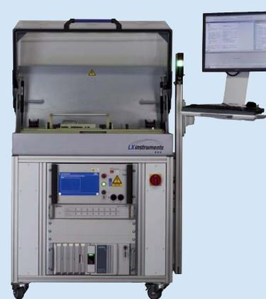
LXInstruments has an integrated test system on display, which allows both: functional tests and safety tests by exchanging the DUT nest. Its advantage is the product contacting which is automatic, safe and repeatable. So far, LXInstruments offers all solution possibilities for the separate as well as the joint functional and safety test: single, separate stations; combined stations with relay switching and combined stations with mechanical switching.
