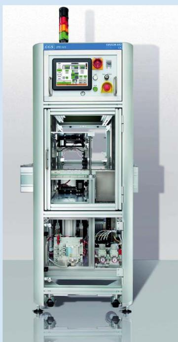
Munich-based CGS showcases the most compact single-head inspection system, the inline test station ITS 115. It processes the multiple PCB-format N5 (max. 175 mm x 175 mm) and offers up to 1,000 contact needles, randomly placeable on upper and lower side. In addition, electrical
